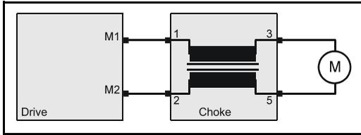
The two cables between the drive and the choke are a source of noise. The cables should be kept as short as possible (300mm is recommended).
