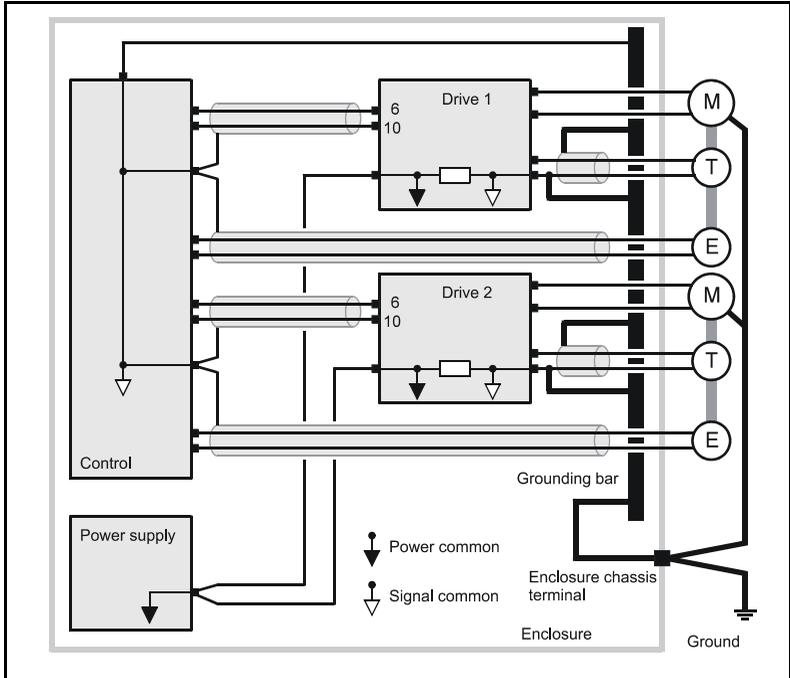
**NOTE** Signal cables and supply cables must be segregated and wired through different trunking
