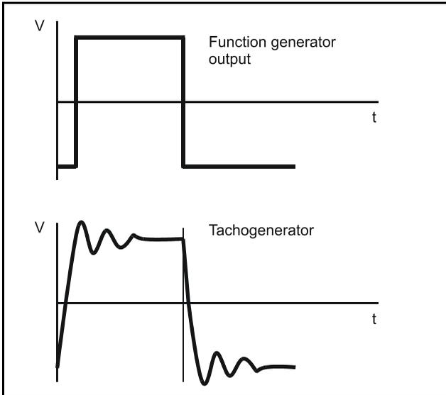
11. The waveform could be as shown in Figure 4-3. In this case, the system has insufficient dynamic gain. Turn the PROPORTIONAL potentiometer clockwise to obtain a waveform without oscillation.
