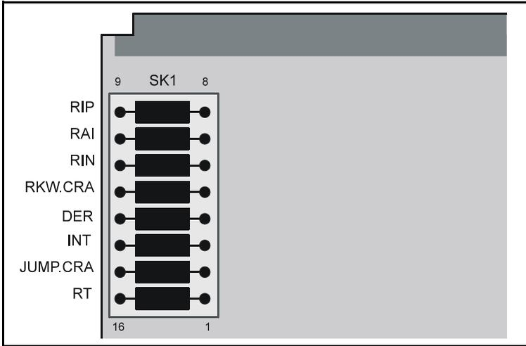
The following resistors and capacitors are mounted on socket SK1:
