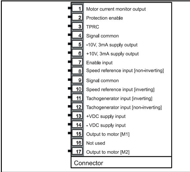
Figure 3-2 Signal and power connections on the 2MH installation kit
