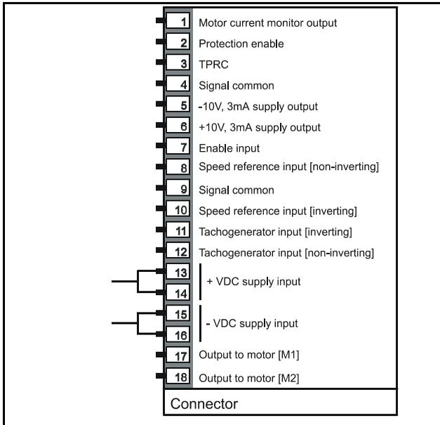
**Figure 3-3 Locations of the signal and power connections on the installation kits**
