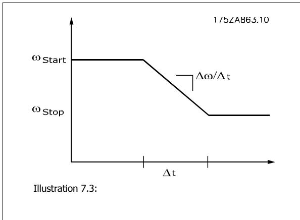
$\Delta t$  is determined by the ramp-down time.
