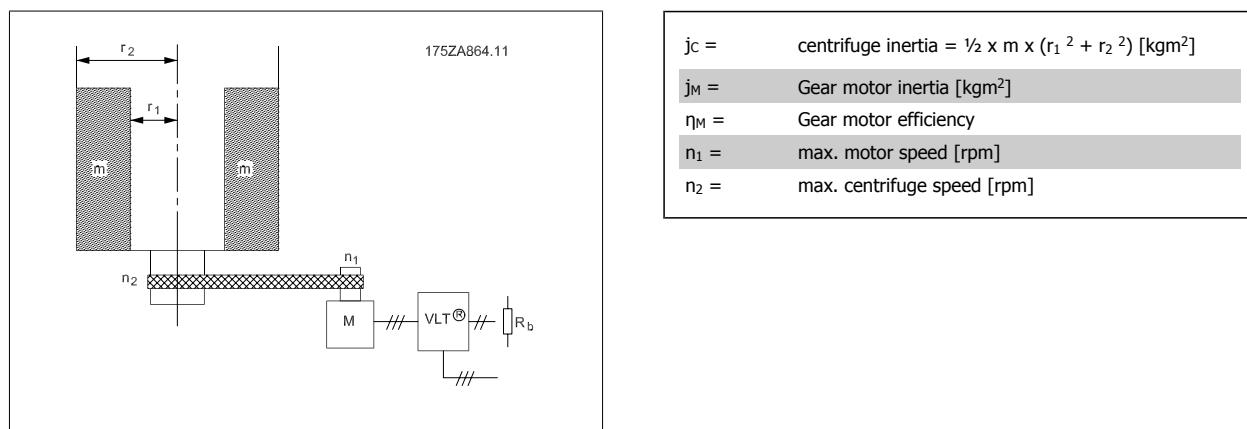
$$E_b = (0.0055 \times j_c \times n_2^2 + 0.0055 \times j_M \times n_1^2) \times \eta_M [\text{Ws}]$$
