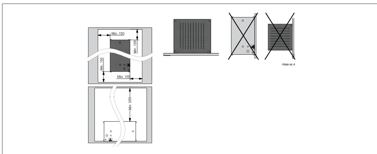
Mounting the resistor so the lamellas are horizontal will cause overheating of the resistor.
