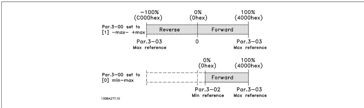
The actual reference [Ref. %] in the VLT frequency converter depends on the settings in the following parameters:
