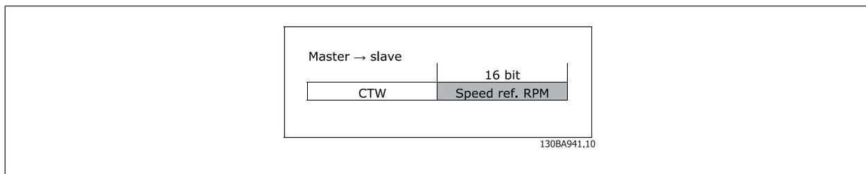
The speed reference value should be transmitted to the VLT frequency converter in the form of a 16-bit word. The value is transmitted directly in RPM.
