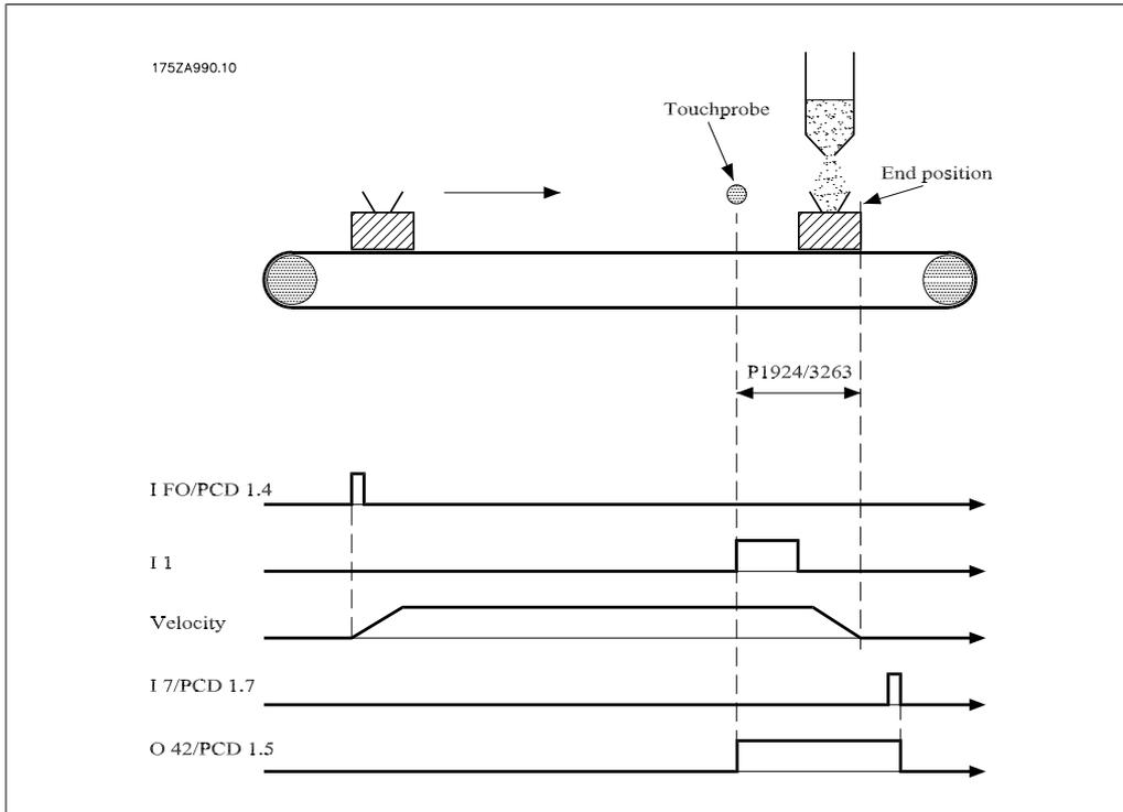
Input 10 is the latch reference index input in digital control mode. PCD 1.4 is the latch reference index input in fieldbus control mode.
