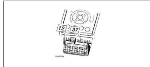
Illustration 1.1: Bridge jumper between terminal 37 and 24 VDC
