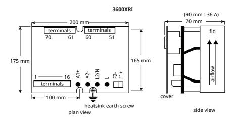
Figure 1 Mechanical dimensions
