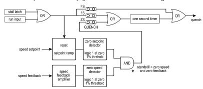
Figure 8 Drive quench circuit
