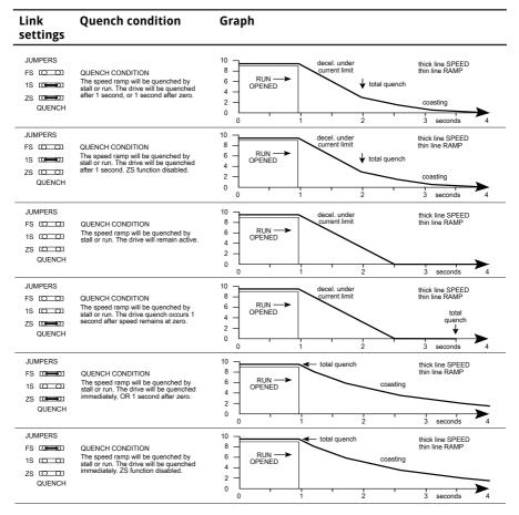
**Quench behaviour is different when using the START/JOG controls on T13/T14 to stop the motor.** Opening the STOP contact on T8 de-energises RL2, disconnecting the ramp circuit from T3, and connecting it instead to XIP on T64 causing the speed to ramp to zero at the set rate. The graph below shows the effect of operating the stop button with just the ZS link in place.
