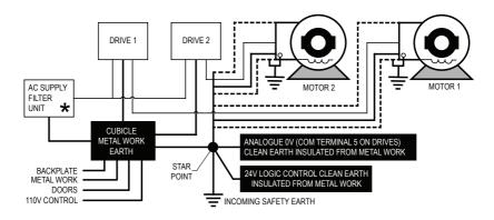
Figure 2 Star point connections for multiple drives
