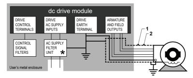
Figure 3 Connections for EMC compliance
