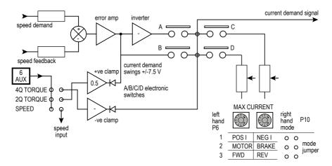
The 2Q TORQUE clamp operates in 1Q and 2Q on the positive current only.
