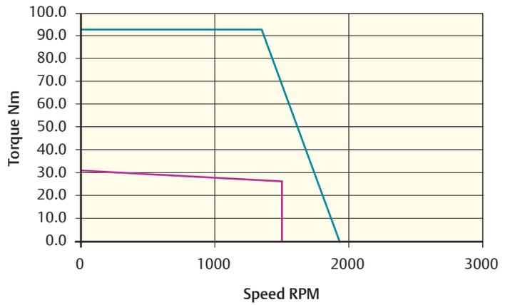
Peak torque (Nm) = 94.50 Stall torque (Nm) = 31.50 Rated torque (Nm) = 27.00
