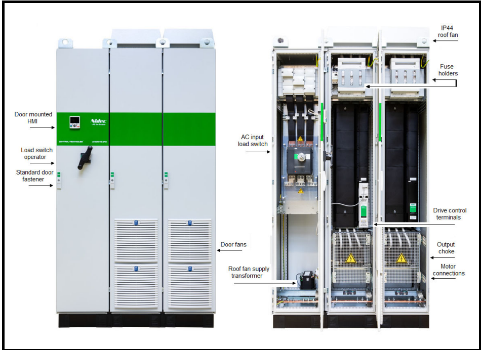
Figure 2-7 Features of the DFS2 cubicle
