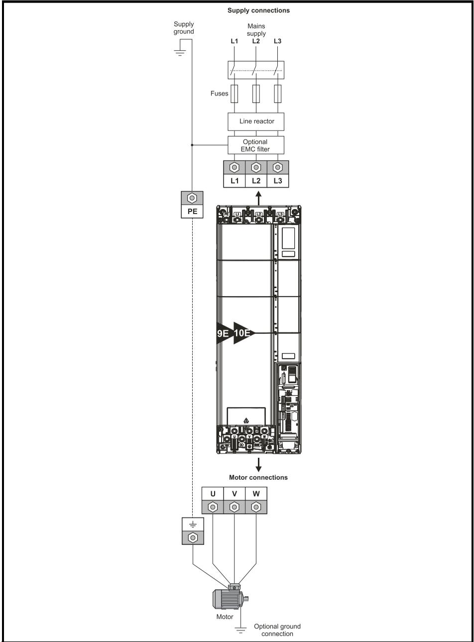
**Figure 6-7 Size 9A power and ground connections**
