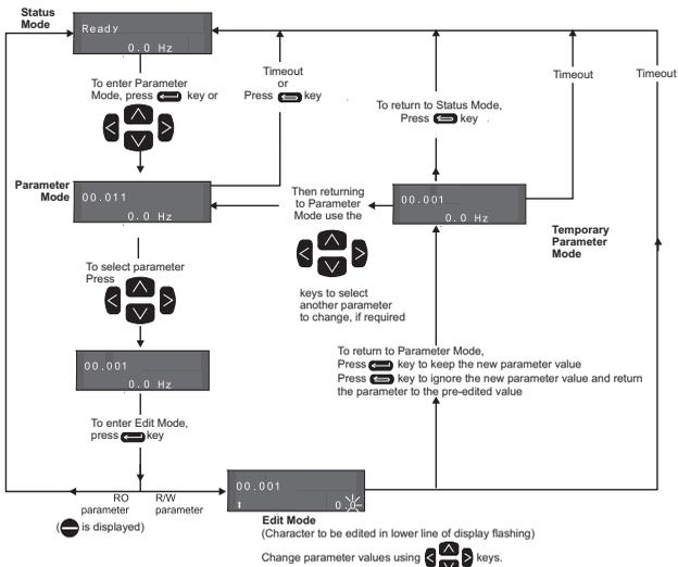
The default status display shows the drive status, the Pump software status and the motor Frequency or Speed.
