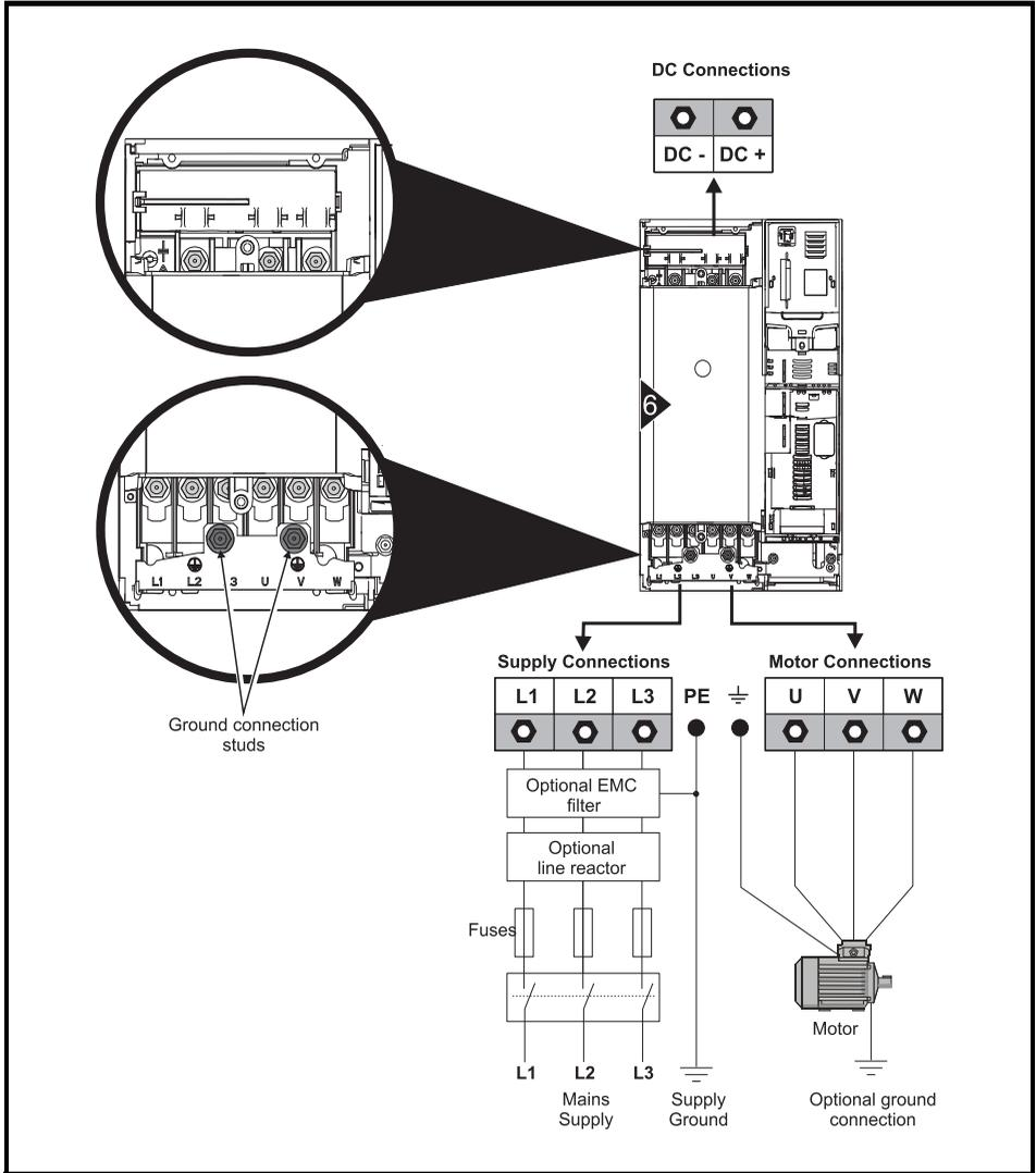
**Figure 6-5 Size 7 and 8 power and ground connections (size 7 shown)**
